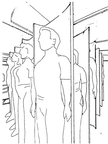
Figure 1: Illustration of standing cabin in a pattern filed by Airbus [7]
