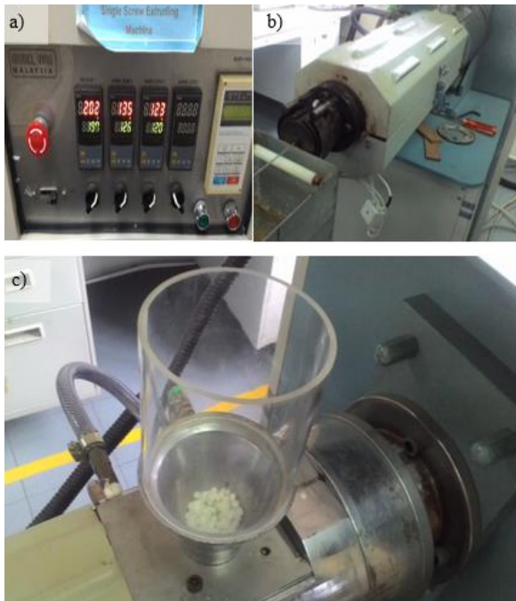
Figure 6: a) Temperature and screw speed control panel b) Heating barrel and extrusion die c) Hopper
