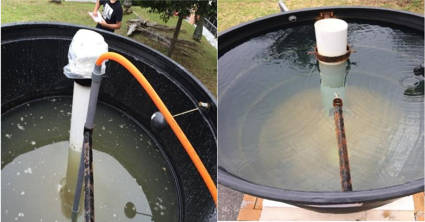
Figure 6 and 5: The clarity of solar pond before and after the particles settle down to the bottom of the pond.
