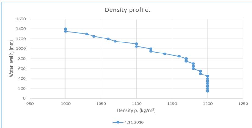
Figure 3: Density profile after establishment of salinity gradient.
