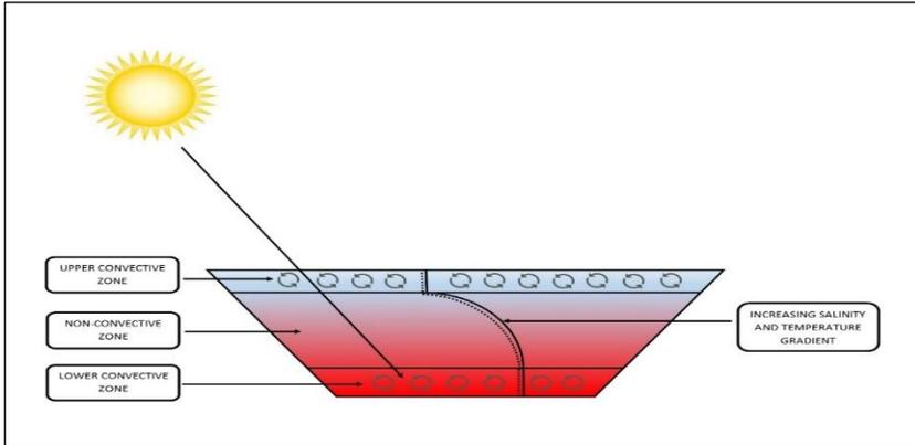
Figure 1: Salinity gradient solar pond diagram.
