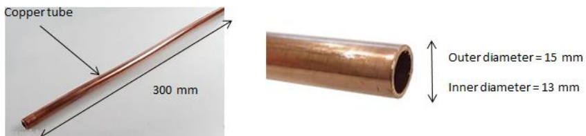
Figure 1: The dimension of the fabricated heat pipe.
