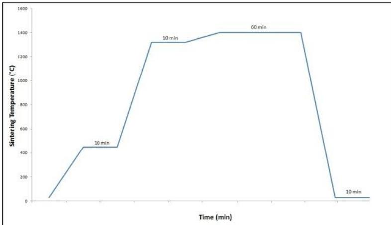
Figure 1. Sintering schedule for WC-Co composite.
