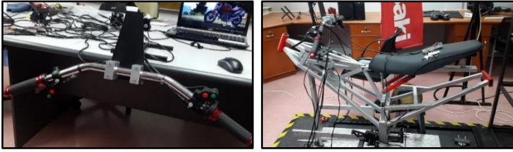
Figure 9: Hs1 Full throttle Motorcycle Controller mounted
