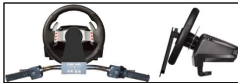
Figure 3: Concept of modifying the MOMO Wheel with a handlebar
