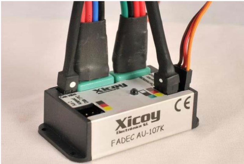
Figure 8: Ports on FADEC ECU
