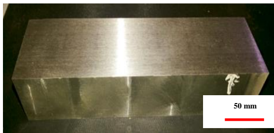
Figure 1: Specimen of Inconel 718
