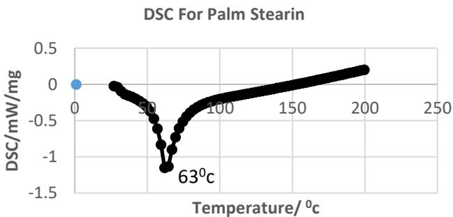
Figure 2(b): DSC plot for Palm Stearin
