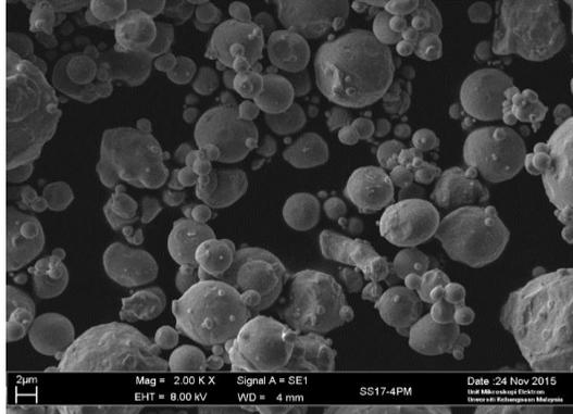
Figure 1(a): SEM Micrograph of 17-4PH
