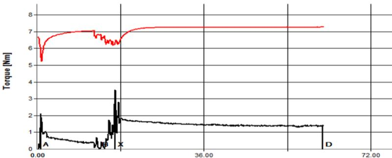
Figure 5(b): Mixing torque evolution versus time for 3YSZ
