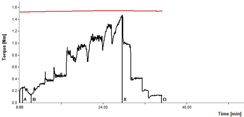
Figure 4(a): Torque evolution related to time for SS17-4PH.
