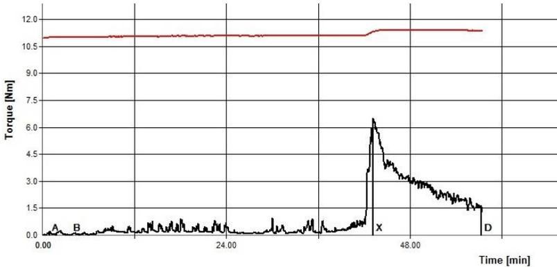
Figure 4(b) Torque evolution as a function of time for 3YSZ.
