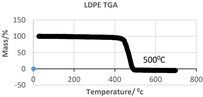
Figure 3(a): Mass decomposition versus temperature profiles for LDPE
