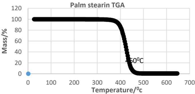
Figure 3(b): Mass decomposition versus temperature profiles for PS
