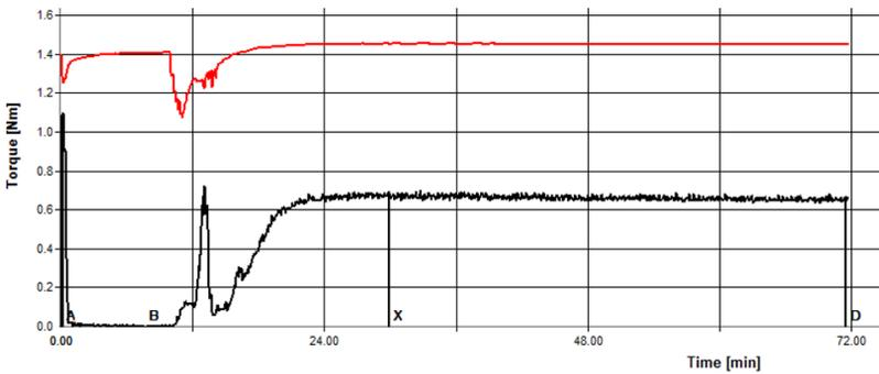
Figure 5(a): Mixing torque evolution as a function of time for SSI7-4PH
