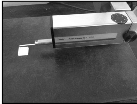
Figure 3: Surface analyzer for measuring surface roughness (Perthometer S2 PGK)
