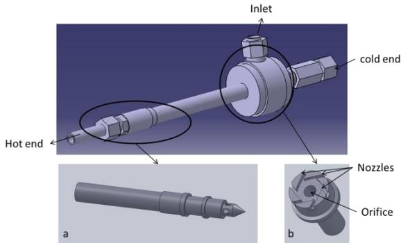
Figure 1: (a) Conical valve and (b) Swirl generator in RHVT
