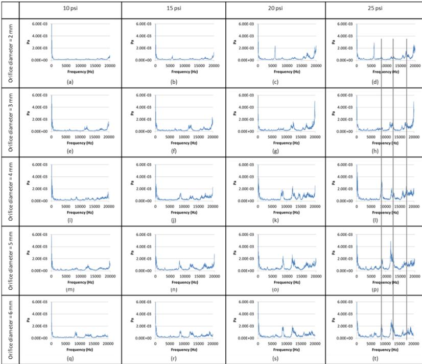
Figure 8: Frequency representation produced for different orifice diameter.
