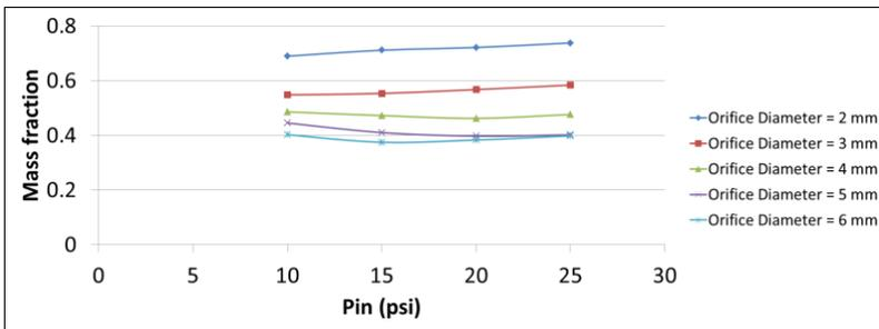
Figure 6: Hot mass fraction vs inlet pressure
