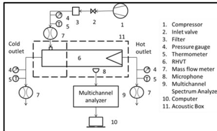
Figure 2: Schematic diagram of the experimental setup
