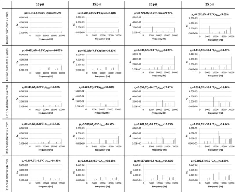
Figure 9: Acoustic signature produced for each different temperature and inlet pressure
