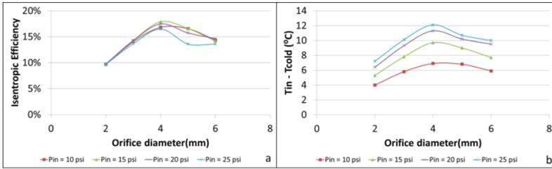
Figure 5 (a): Orifice diameter vs isentropic efficiency (b): Orifice diameter vs temperature difference
