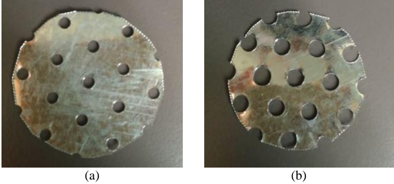
Figure 6: Perforated panel, (a) 3 mm perforation diameter, (b) 4.5 mm perforation diameter.
