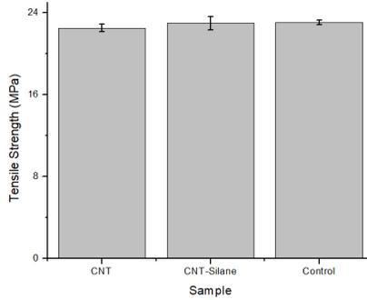
Figure 2: Tensile strength of CR compound samples
