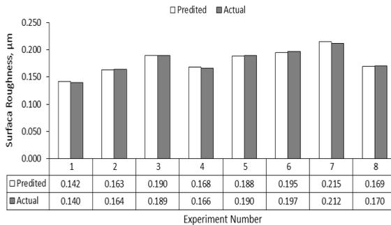
Figure 3: Comparison between actual and predicted Ra
