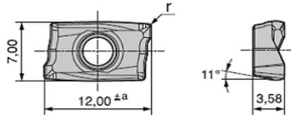
Figure 1: DLC coated cutting tool dimensions in mm
