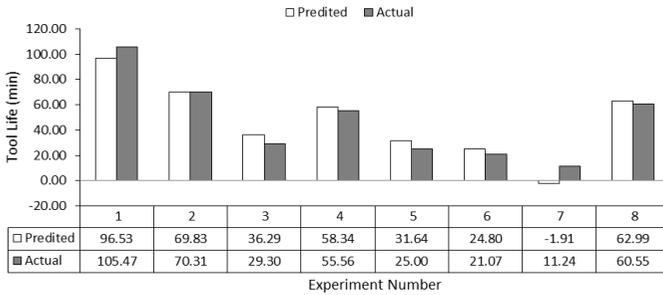
Figure 6: Comparison of actual vs predicted tool life
