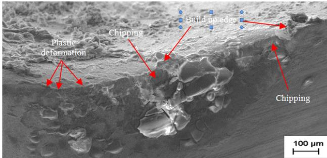
Figure 9: SEM images of a worn out view on the flank face for DLC coated carbide insert at cutting speed 350 m/min, feed rate 0.04 mm/tooth and radial depth 25 mm in dry cutting condition.
