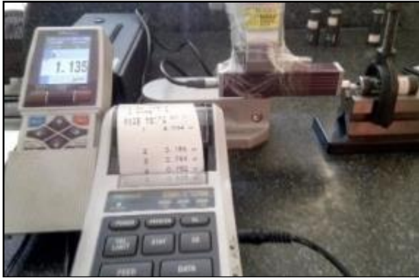
Figure 4: Set up for surface roughness measurement
