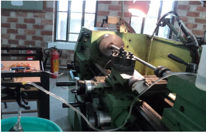
Figure 4: Cooling control panel setup on center lathe machine
