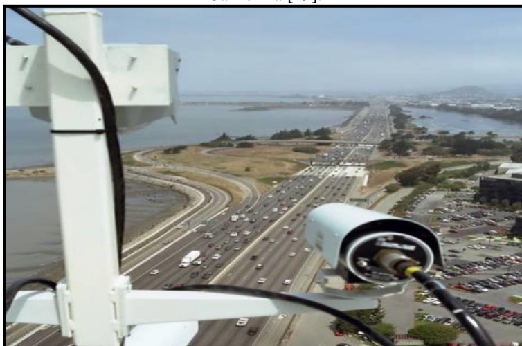
Figure 2: A video camera that overlooks I-80 is recording vehicle trajectory data [19].
