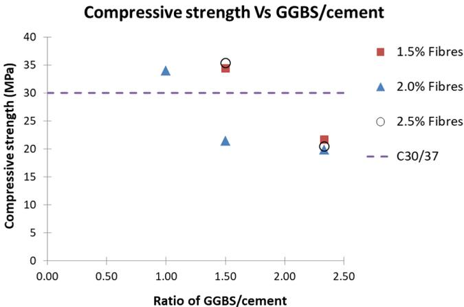
Figure 4: Effect of GGBS/cement ratio in compressive strength.
