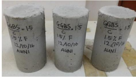
Figure 5: ECC cylinders after compression test.
