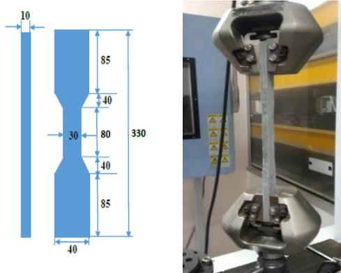
Figure 3: Tensile test.
