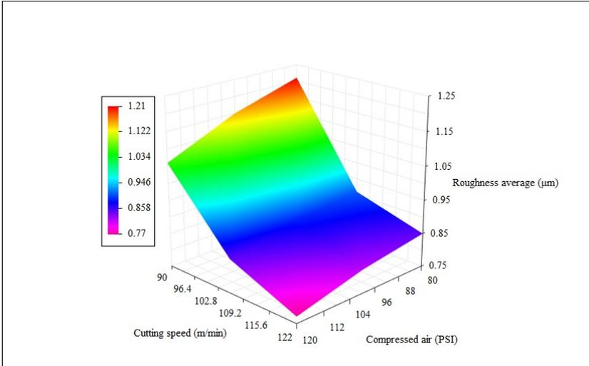
Figure 3: Surface plot of the relationship between cutting speed, compressed air, and roughness average
