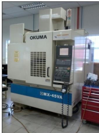
Figure 1: Okuma MX-45VA vertical CNC machining centre
