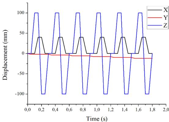
Figure 6 : Tool movements in 2 mm of step down
