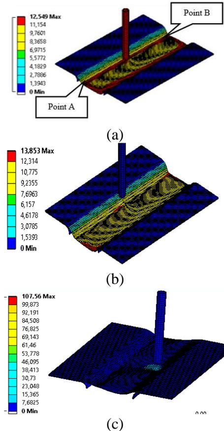
Figure 8 : SPIF simulation results of step down; (a) 2 mm; (b) 4 mm; (c) 6 mm
