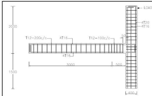
Figure 3: Detailing of corner beam-column joint.
