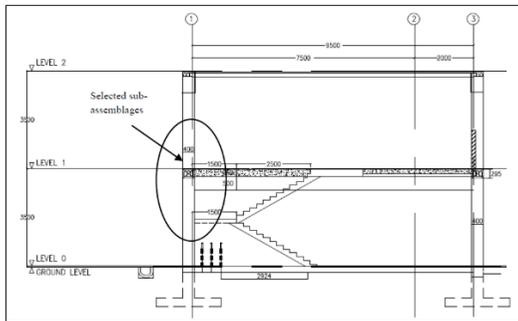
Figure 2: The location of corner beam-column joint at two-storey school building.
