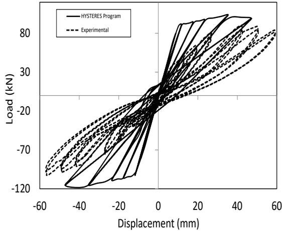
Figure 8: Comparison of hysteresis loops between experimental and modeling.
