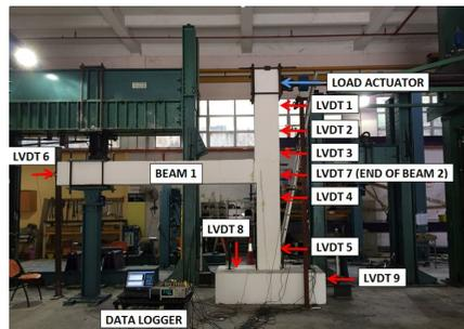
Figure 4: Experimental set-up of corner beam-column joint
