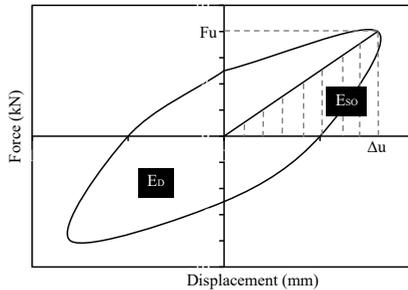
Figure 6: Hysteresis loop with indication of energy dissipation ( $E_D$ ) and strain energy ( $E_{so}$ ).
