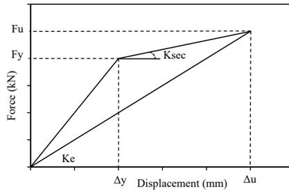
Figure 7: Differences between  $K_{elastic}$  and  $K_{secant}$ ,
