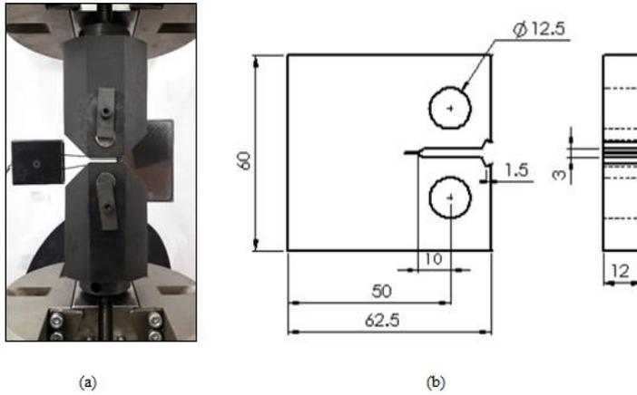
Figure 3: (a) Experimental setup for FCG rate test, (b) Specimen geometry used for FCG rate test (all dimensions are in millimeters)
