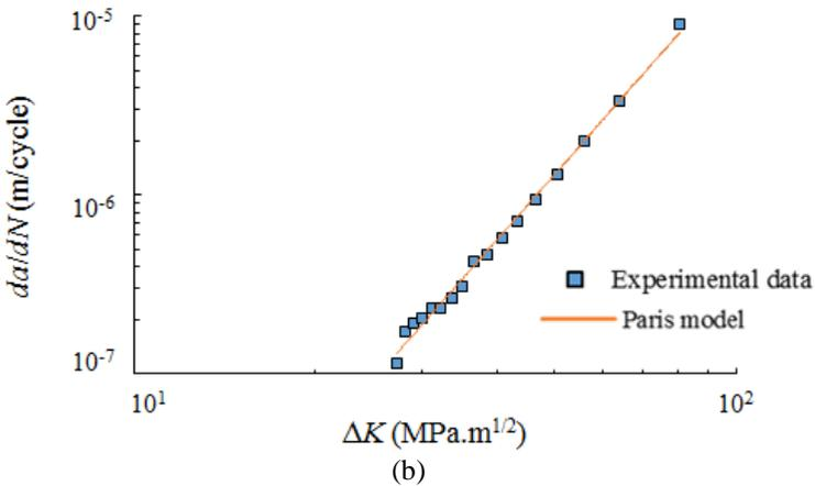
Figure 8: Fatigue crack growth curve described by the Paris model of (a) as-received and (b) dual-phase steels.
