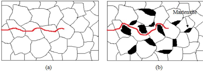
Figure 1: Schematic of crack path in ; (a) as-received steel and (b) dual-phase steel.
