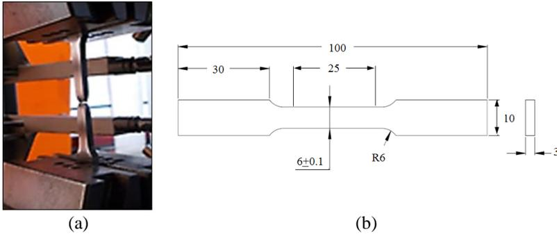
Figure 2: (a) Experimental setup for tensile test, (b) Specimen geometry used for tensile testing (all dimensions are in millimeters).
