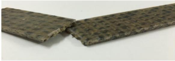
Figure 8 (b): KES composite specimen that is fractured after tensile test
