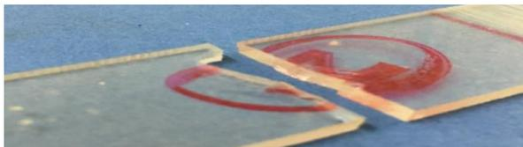
Figure 9 (b): Epoxy specimen that is fractured after tensile test
