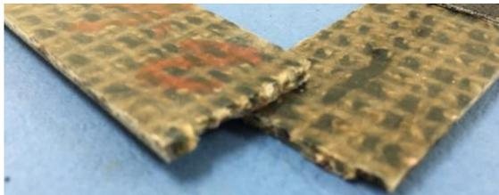
Figure 7 (b): KE composite specimen that is fractured after tensile test
