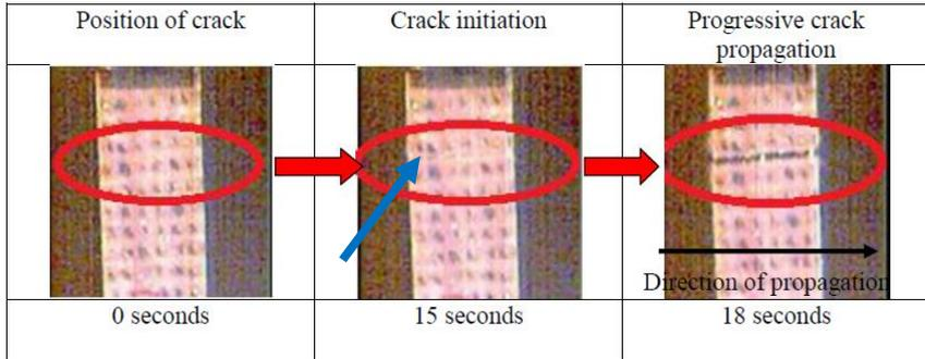
Figure 12 Crack propagation as observed using a high speed camera
