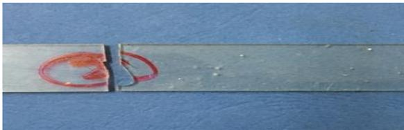
Figure 9 (a): Epoxy specimen failed at gage length
