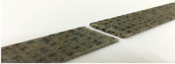
Figure 8 (a): KES composite specimen failed at gage length
