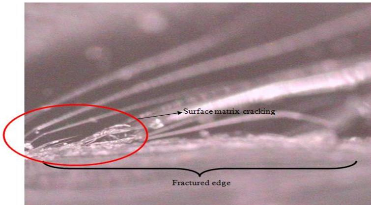
Figure 13: Surface matrix cracking of pure epoxy specimen on fractured edge ( $10\times$  magnification)
