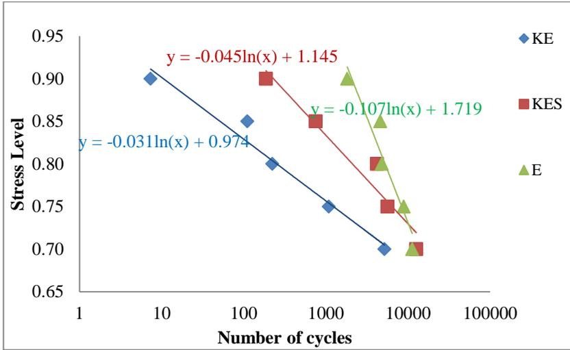
Figure 10: S-N curve for all specimens
