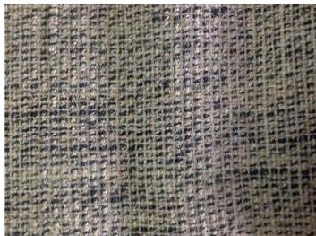
Figure 1: Woven kenaf fiber used for research study
