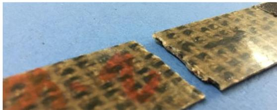
Figure 7 (a): KE composite specimen failed at gage length
