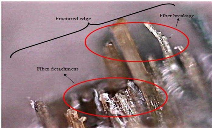
Figure 14: Fiber breakage and detachment can be observed on the fractured edge of KES specimen (10 × magnification)
