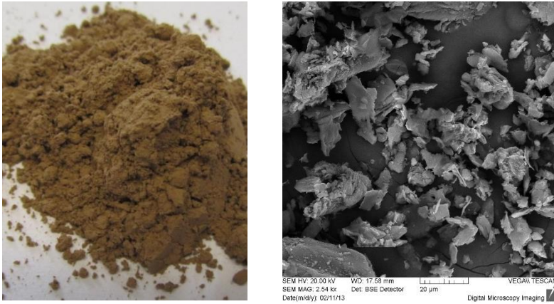
Figure 3: Coconut particles after cryogenic grinding (left) and SEM image of coconut particles after cryogenic grinding (right)
