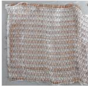
Figure 2: Actual sample of 3DAI woven fabric
