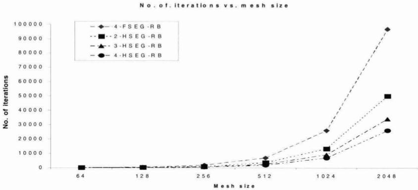
Figure 5: Number of Iterations Versus Mesh Size of the 4 Point FSEG-RB and HSEG-RB Methods
