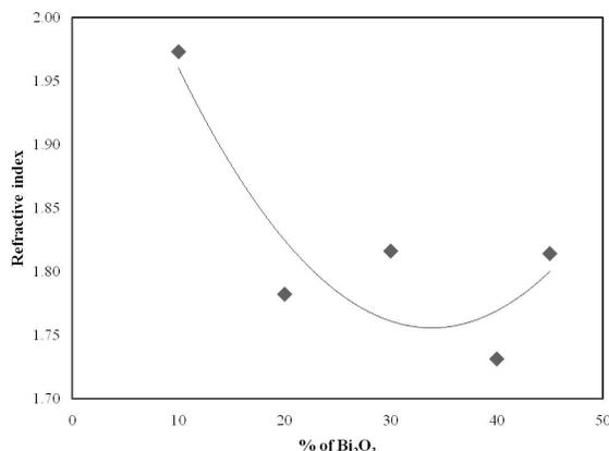
Figure 7: Refractive indices of xBi<sub>2</sub>O<sub>3</sub> - (1-x)ZnO - 0.2B<sub>2</sub>O<sub>3</sub> - 0.3(SiO<sub>2</sub>)RHA glass samples.
