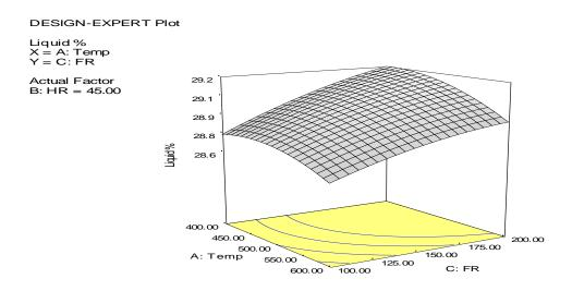
Figure 4: The relationship between the final temperature and gas flow rate to the liquid yield.
