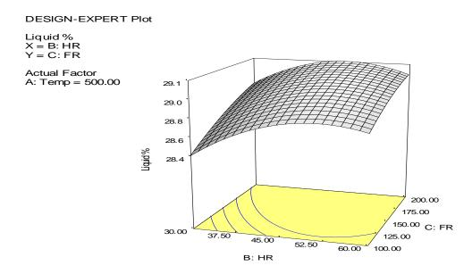
Figure 5: The relationship between the heating rate and gas flow to liquid yield.
