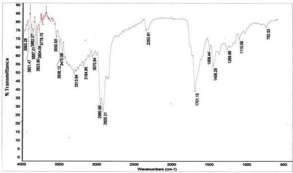
Figure 6: FT-IR spectra of the bio-oil
