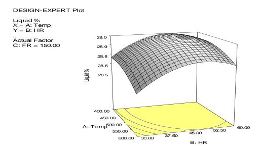
Figure 3: Relationship between effect of final temperature and heating rate on the liquid yield.
