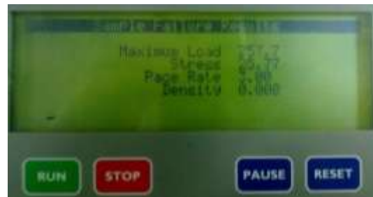
Photo 4 Strength reading from compressive strength test machine
