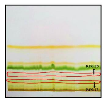
Figure 1 pTLC of Antioxidative compound (R<sub>f</sub> 0.17) of DCM extract of *L.indica* stem marked on pTLC
