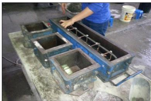
Figure 3. Steel mould used for the cube and beam samples
