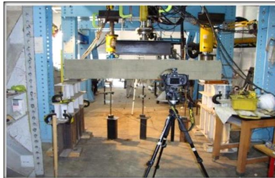
Figure 5. The camera setup and LVDT installation of the work
