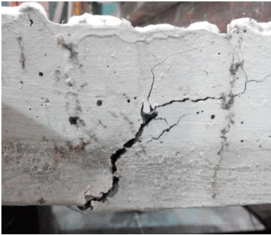
Figure 9: Crack Pattern of Failed Two-Ribbed Slab (source by author)
