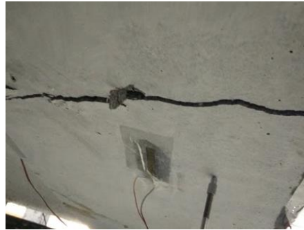
Figure 9: Crack Pattern of Failed Two-Ribbed Slab (source by author)
