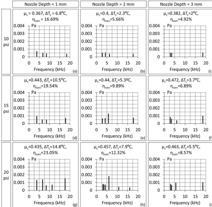
Figure 14. Frequencies signatures for different inlet pressure using different nozzle depth (cold tube)
