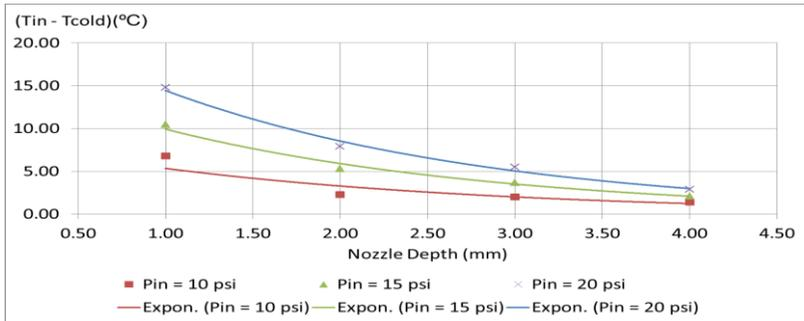
Figure 6: Variation of temperature difference between the inlet and the cold outlet with nozzle depths for three inlet pressures
