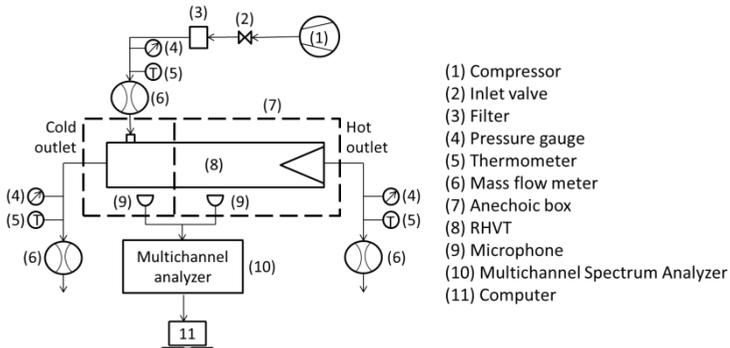
Figure 2: Experimental setup schematic diagram
