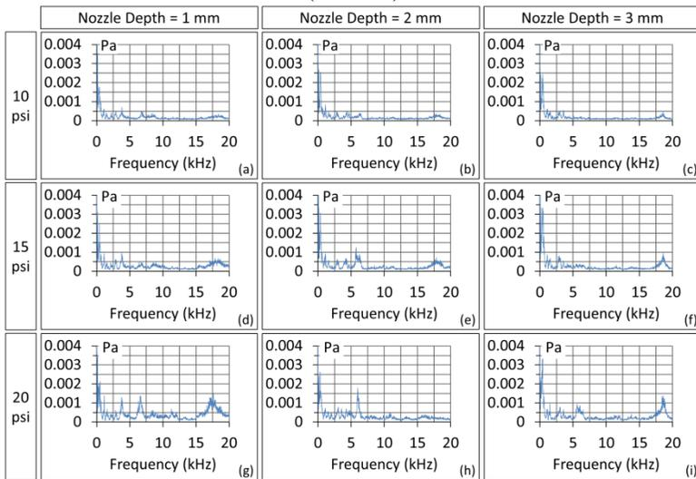
Figure 11. FFT results for different inlet pressure using different nozzle depth (cold tube)
