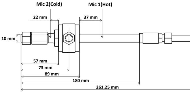
Figure 3: RHVT dimension and microphones location
