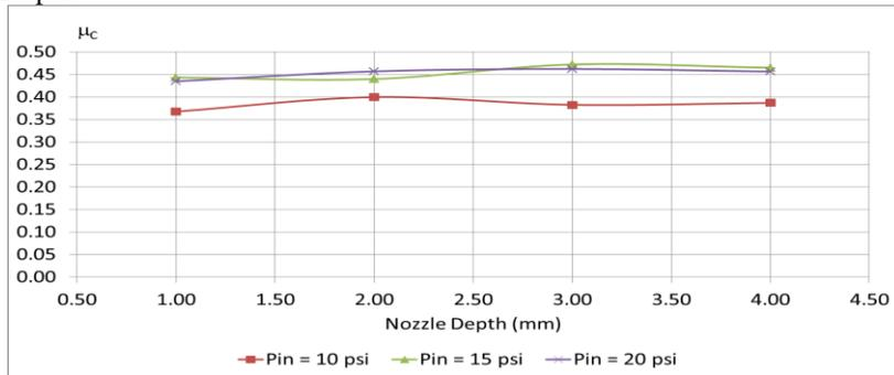
Figure 5: Variation of cold mass fraction with nozzle depths for three inlet pressures
