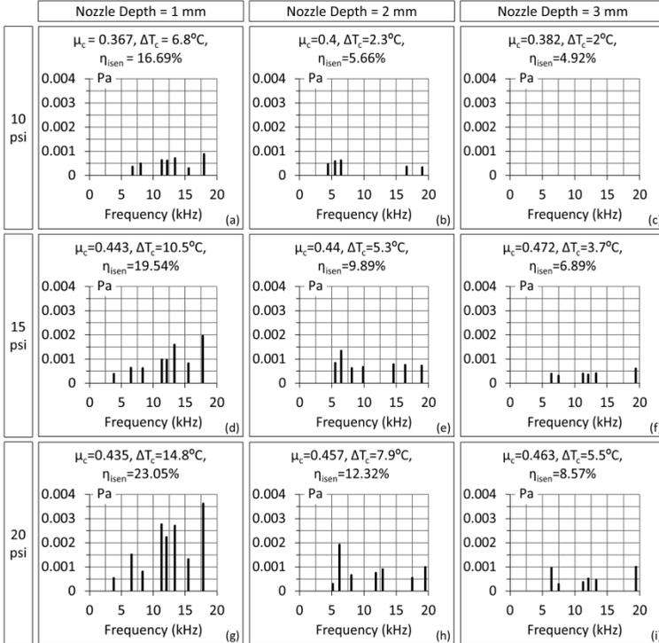
Figure 13. Frequencies signatures for different inlet pressure using different nozzle depth (hot tube)
