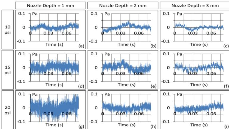
Figure 8: Time representation of sounds recorded for different inlet pressure using different nozzle depth at hot tube
