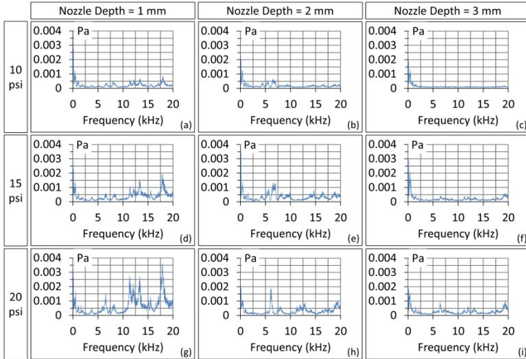
Figure 10. FFT results for different inlet pressure using different nozzle depth (hot tube)
