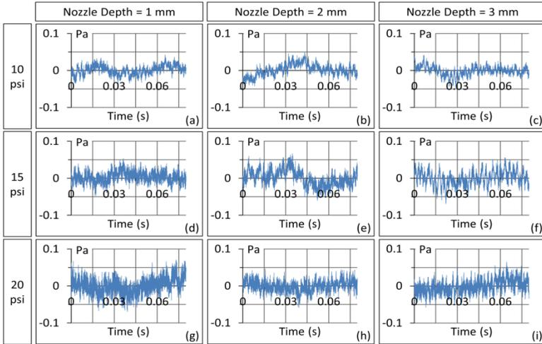
Figure 9: Time representation of sounds recorded for different inlet pressure using different nozzle depth at cold tube
