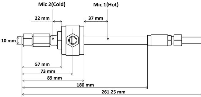
Figure 3: RHVT dimension and microphones location
