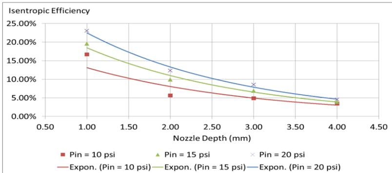
Figure 7: Variation of isentropic efficiency with nozzle depths for three inlet pressures
