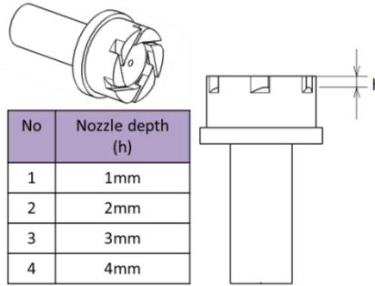
Figure 4: Swirl generator used in the experiment
