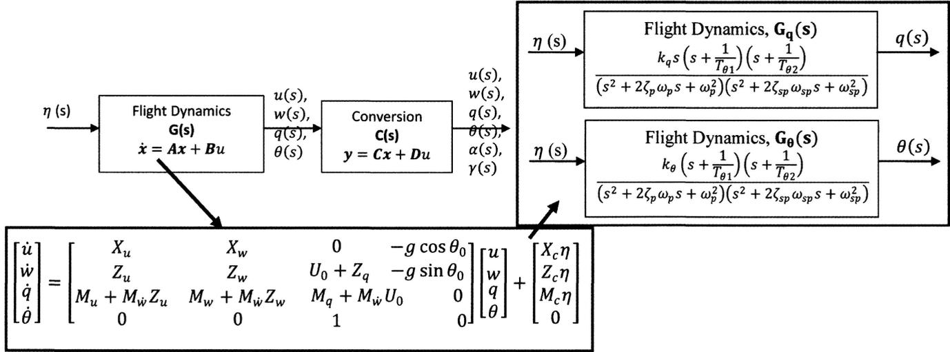
Figure 1: Above - Axes systems, forces, moments, velocities, angular velocities (rates) and angles. Below - Block diagram of Baseline-II E-2 BWB unaugmented longitudinal flight dynamics
