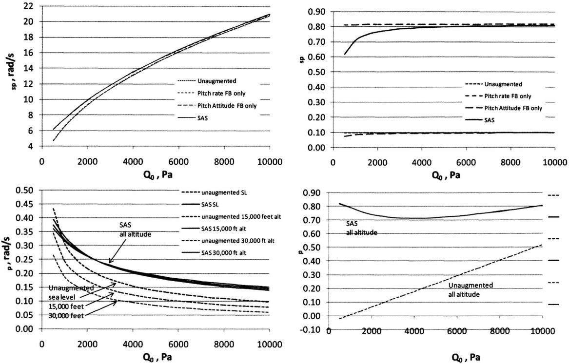
Figure 7: Short-period and Phugoid modes' natural frequencies and damping ratios – comparisons between SAS and unaugmented aircraft.
