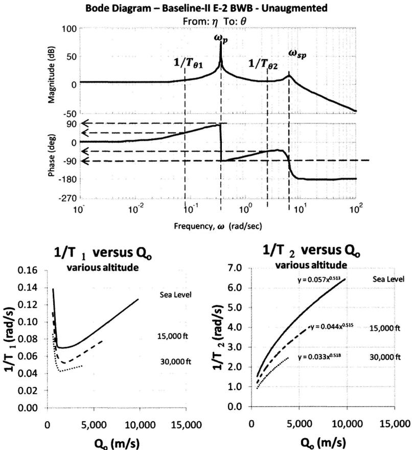
Figure 5: Example of bode plots (magnitude and phase angle of pitch angle  $\theta$  versus canard input frequency  $\omega_c$ ) for unaugmented Baseline-II E-2 BWB longitudinal dynamics and its corresponding phase lead frequencies versus  $Q_0$  for various altitudes.
