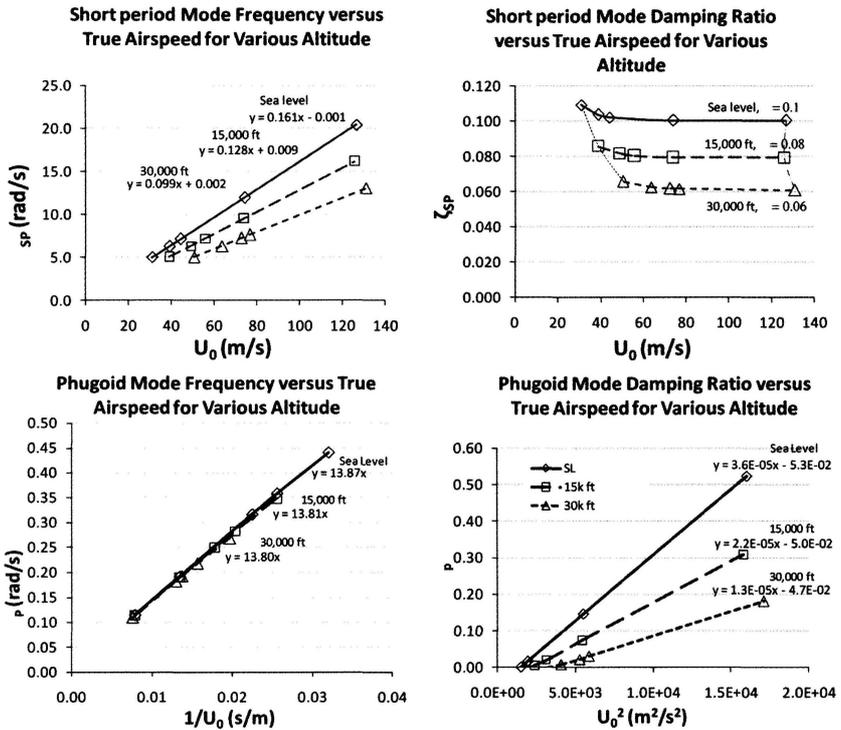
Figure 2: Short period and Phugoid natural frequencies and damping ratios plots against airspeed for various altitudes.
