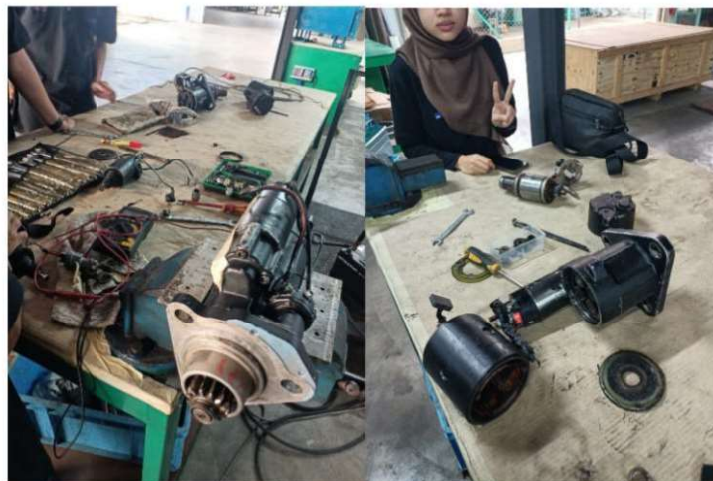
Figure 2: Disassembled Starter Motor Components During the Inspection Process
