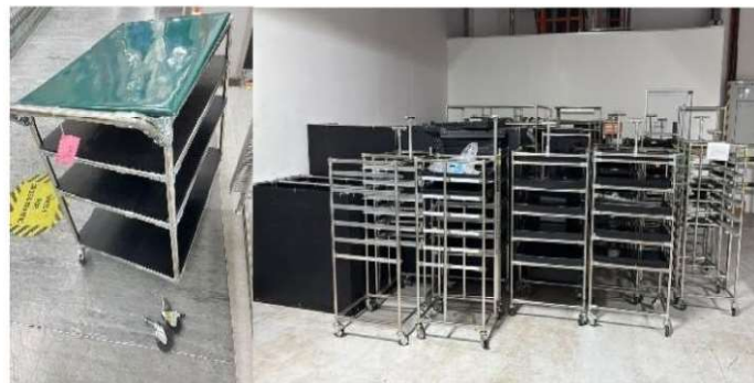
Figure 3: Example of the material trolley that has been fabricated
