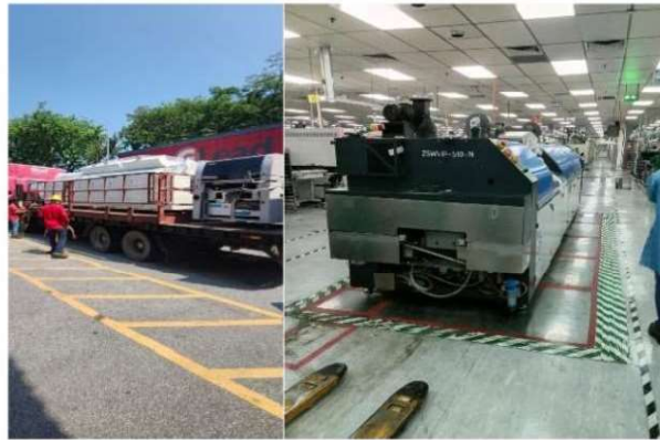
Figure 4: Movement of the Wave Machine from Another Plant to A New Production Line from Left to Right, Respectively
