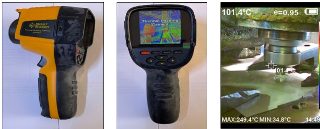
Fig. 5. FSW thermal imaging camera (SMART SENSOR, Model ST9450).
