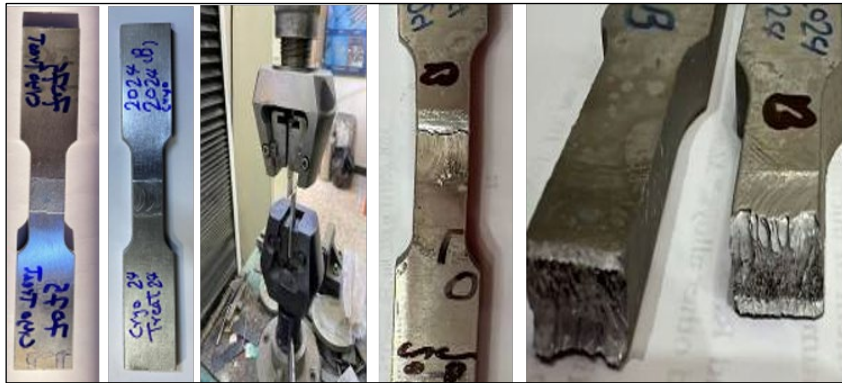
Fig. 14. Fracture surface morphology of FSW joint.
