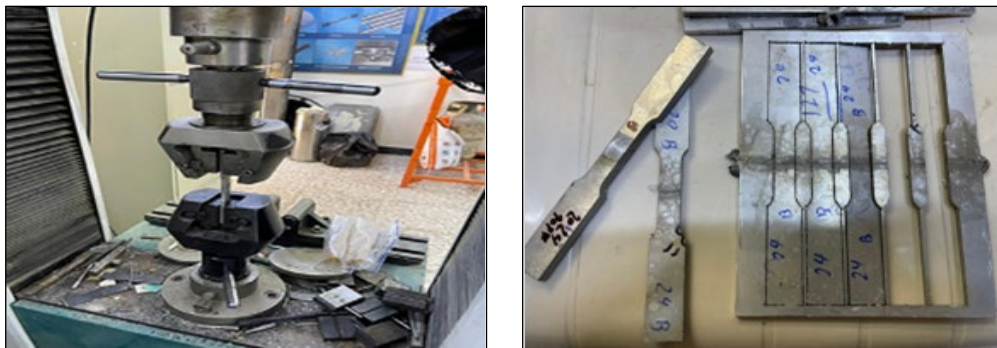
Fig. 7. Tensile testing specimen for FSW joints.
