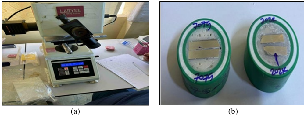
Fig. 8. (a) LARYEE Vickers microhardness testing machine and (b) epoxy resin mold.
