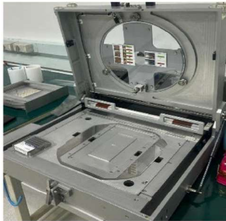
Figure 3: Mounting Tape Machine
