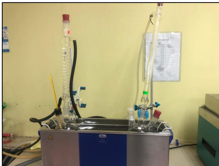
Experiment Set-up for Enzymatic Transesterification in Ultrasonic System
