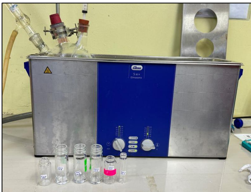
Experimental Set-up for Initial Reaction Rate Measurement (0–30 minutes) in Biodiesel Synthesis Using Immobilized CALB
