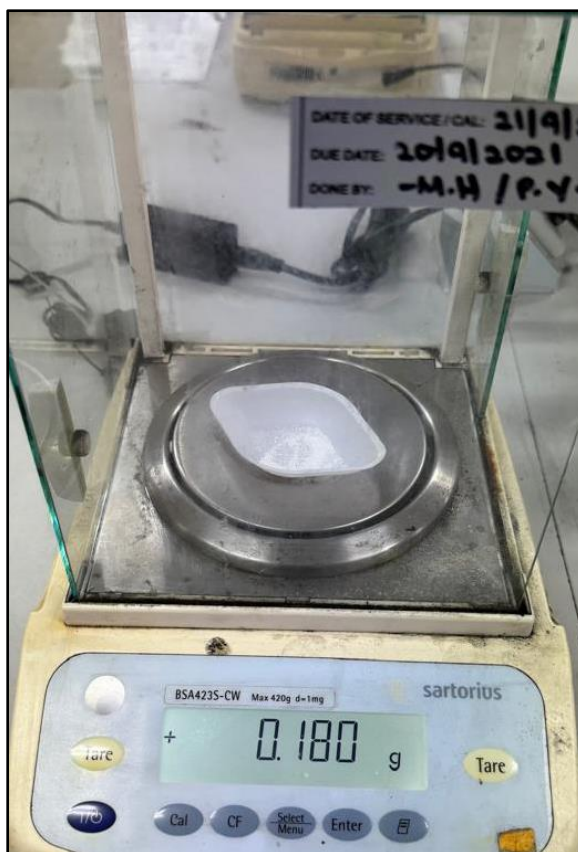
Weighing of 0.18g of Immobilized Lipases for the Transesterification Reaction Experiment
