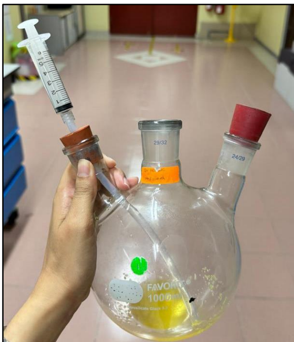
Three-neck Flask Set-up Containing WCO, Methyl Acetate, Lipase, Prepared for the Transesterification Reaction Experiment.
