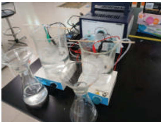
Figure 1. The actual electrocoagulation process experimental set-up
