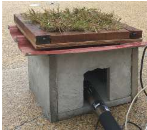
Figure 1: Green Roof with 3D Concrete House Model
