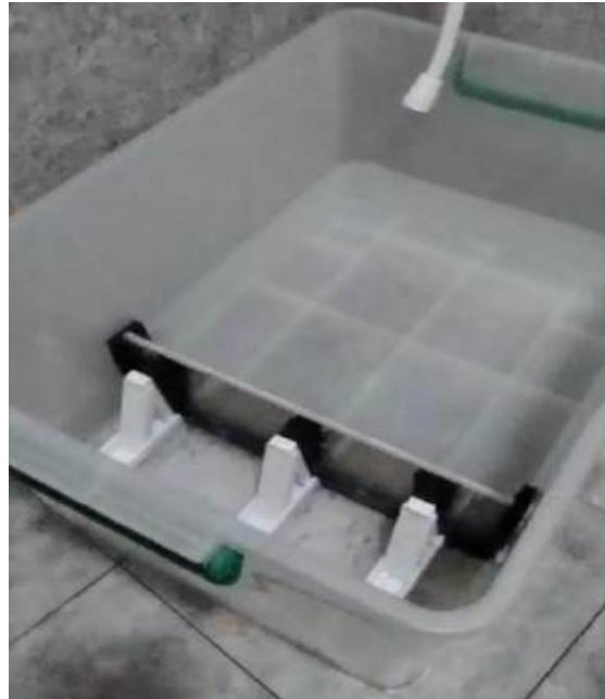
Figure 3. Prototype of the flood barrier
