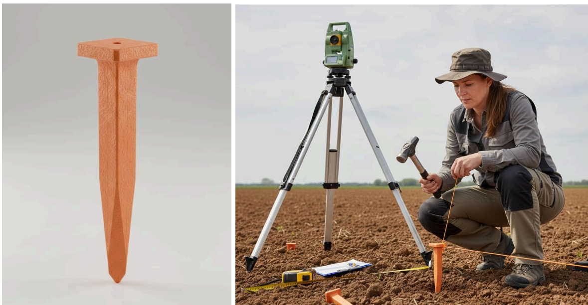
Figure 3.3.4.2 and 3.3.4.3 : 3D Illustration of Eco-Peg™ Model and surveyor using on the site
