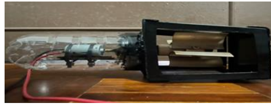
Figure 2. Side view of Compact Hydro Vertical axis Blade Turbine
