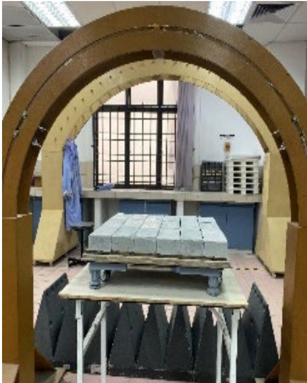
Fig. 5. NRL Free Space Arch measurement setup.
