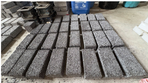
Fig. 3. Brick curing process
