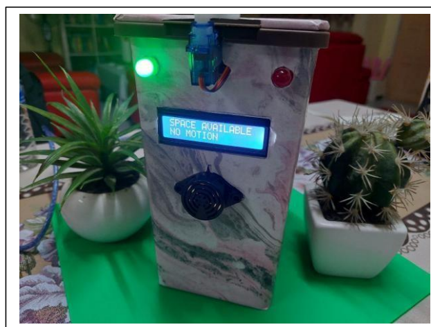
Figure 4.2: LCD Displays "Space Available and No Motion"
