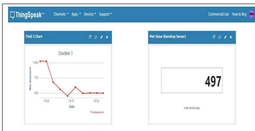
Figure 4.8: ThingSpeak Channel Analysis Shows the Moisture (wetness) Level inside the Dustbin. The threshold is set to number 300
