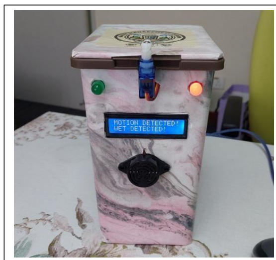
Figure 4.4: LCD Displays the Moisture Level Detection
