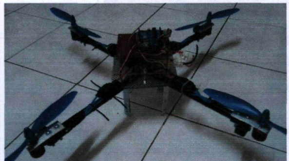
Figure 7: The overall Quad-Copter hardware with Arduino UNO R3 controller board.
