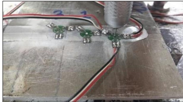
Fig. 6. Central drilling test (for residual stress test).
