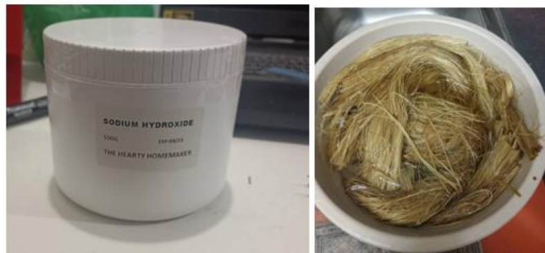
Figure 3: Treat banana fibre with NaoH
