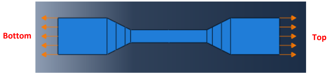
Figure 12. Boundary Condition of part in Top and Bottom
