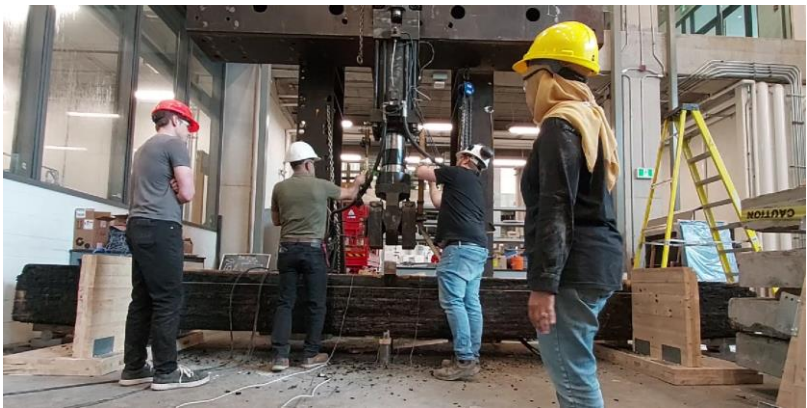
Figure 4 : While conducting the timber beam bending test
